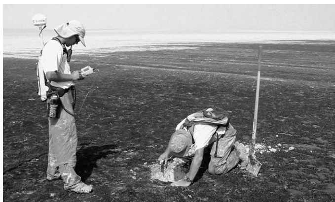
Fig. 1. Field data logging of oiling conditions using a weatherproof hand-held field computer linked to a GPS. Al Musallamiyah, Eastern Province Saudi Arabia, October 2002 (photo by T. Gale, EESA).
